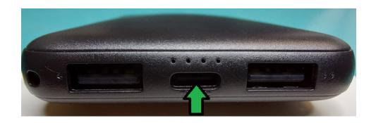
2. After the battery is completely charged, unplug the charging cable from the battery, and use one of the USB Type A ports to supply power to your SkyBridge Max.
